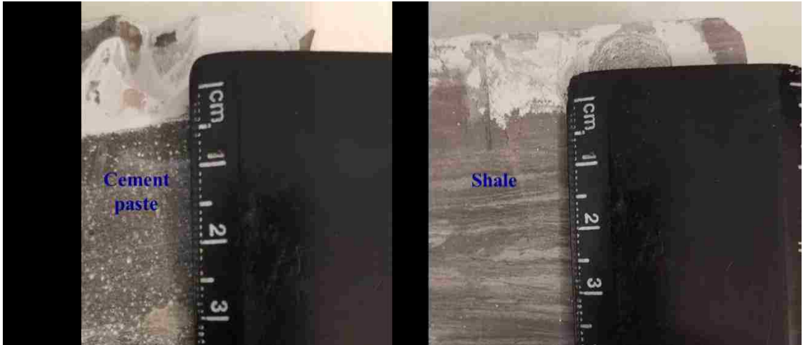
Figure 3.43: Microscopic images of cement-shale interface sealed with microfine cement with two different sides showing depth of microfine cement penetration of cement paste and shale sides.
