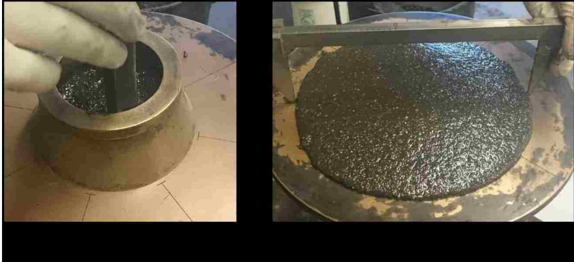
Figure 3.12: (a) Filling the flowability cone (b) taking readings using test caliber.
