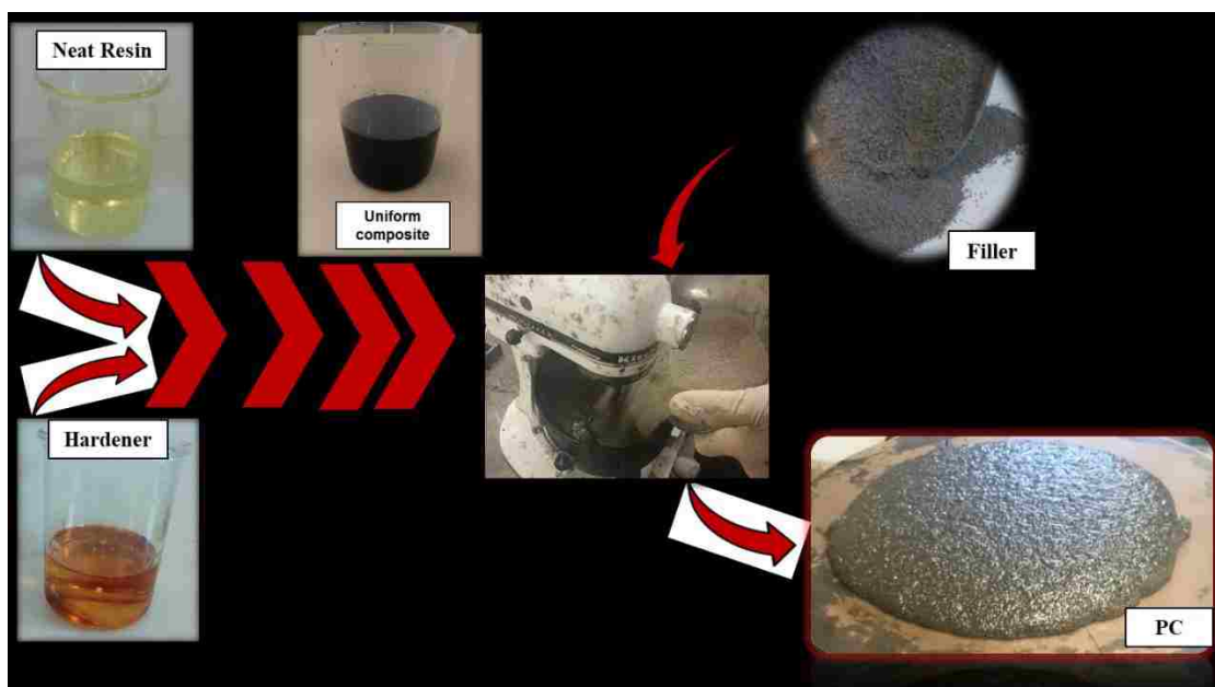
Figure 3.6: Schematic of mixing procedure of polymer-cement nanocomposites.
