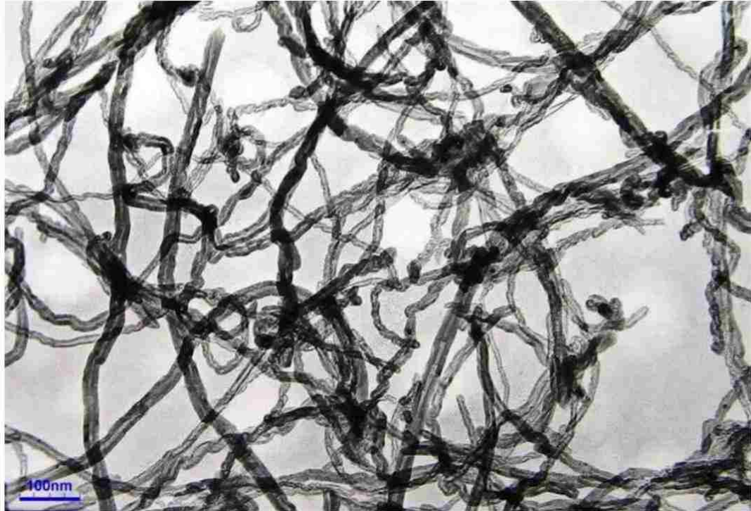
Figure 3.2: Transmission electron microscope (TEM) images of MWCNTs.
